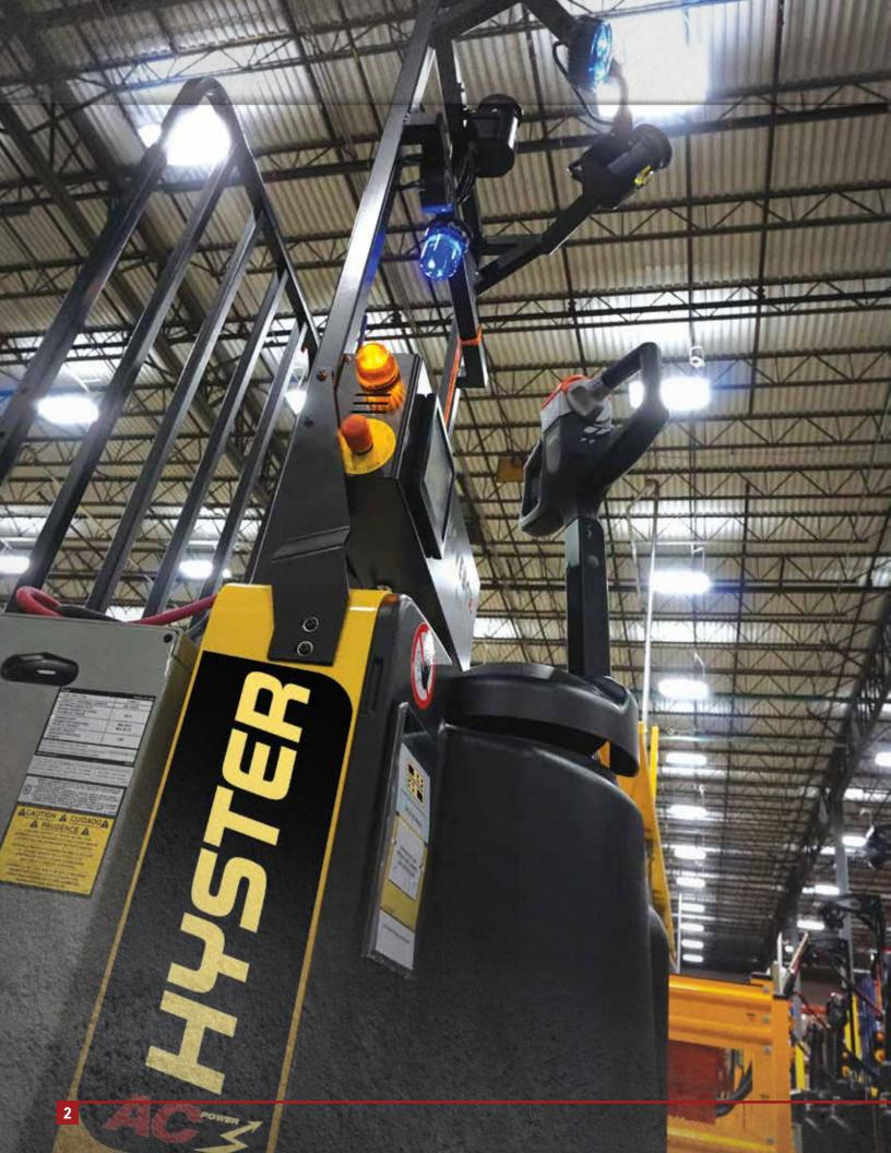
By combining the Hyster<sup>®</sup> End Rider and Tow Tractor with Balyo's navigation technology, the B80Z<sup>HD</sup> and the LO5.0T become robotic lift trucks. The infrastructure-free navigation relies on structural features such as walls, columns or racks, to make the Driven by Balyo technology flexible, scalable, and economical.
